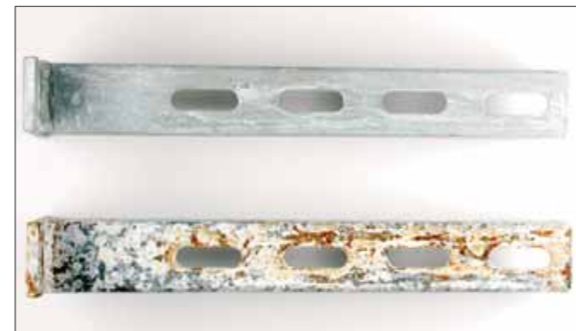
Cantilever Bracket 41/41 after 1,440 h salt spray test; Above: zinc-lamella coated Below: zinc-galvanised
