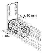
Assembly to Beam Section TP F 80, for instance Cantilever Bracket AK F 80 and others.
